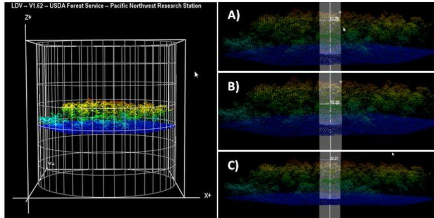
Figura 3. Illustration 3-D LIDAR point clouds in LiDAR Data view in Fusion. A) LiDAR points clouds of plot, B) Mean tree height, C) Minimum tree height and D) Maximum height
