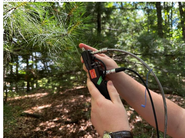
Figure 10 Image of the small leaf adapter attached to the leaf clip taking a scan of a pine needle.
