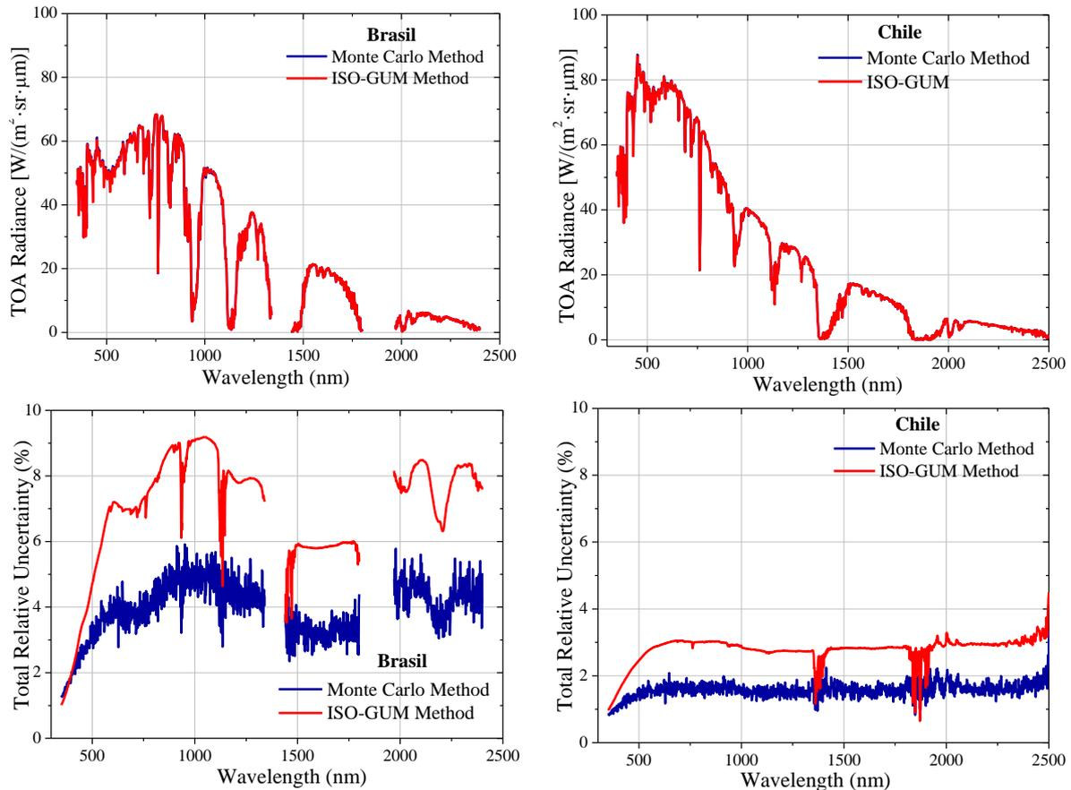
**Figure 5:** In (a) and (b) TOA radiance predicted by MODTRAN; and (c) and (d) its final relative uncertainty (in percentage) using Brazil and Chile sites, respectively.
