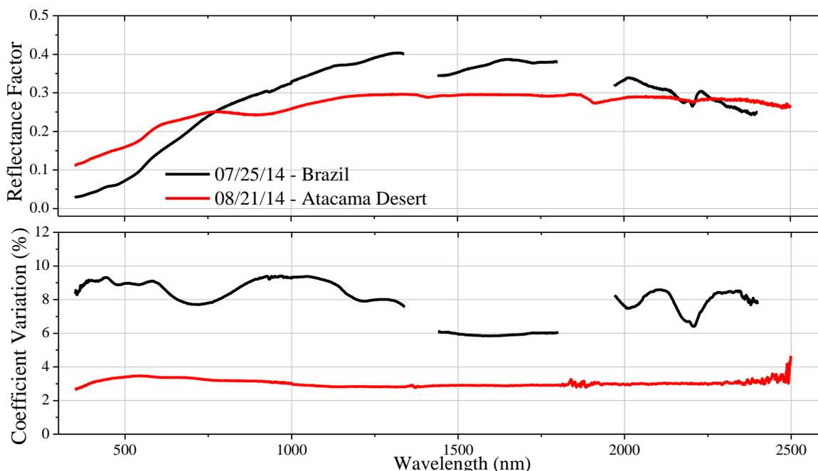
**Figure 1.** In (a) Spectral reflectance results of the reference sites; and (b) surface coefficient of variation in percentage.
