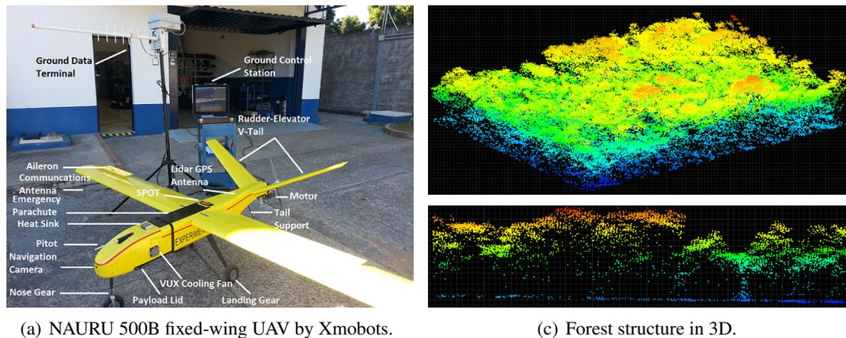
Figure 3: Nauru 500B UAV and Lidar data collect during one of its test flights on Jun 29, 2016 near the city of São Carlos, São Paulo state, Brazil.
