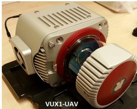
(a) VUX1-UAV Lidar Scanner by RIEGL
