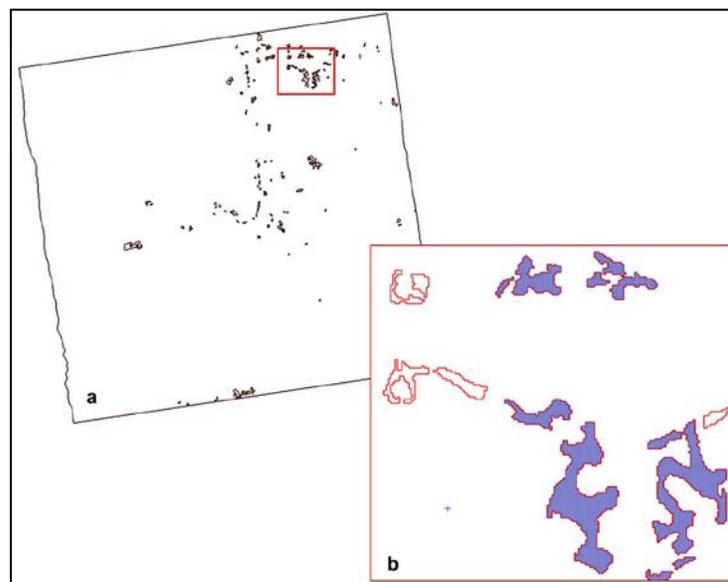
**Figure 3. RADARSAT-2 detected changes between 2011-2012 for the entire image (a) (50 km x 50 km) and (b) a subscene (~ 10 km x 10 km). Based on visual analysis, the blue polygons were categorized as forest harvesting and the red polygons were categorized as false positives.**
