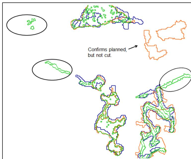
**Figure 4.** This is the same area as Figure 3b. The RADARSAT-2 detected changes are indicated by blue polygons, and overlaid with BCFS cut blocks (orange polygons) and CFS tree loss (green polygons). The BCFS cut blocks not correlated with CFS tree loss and RADARSAT-2 changes were planned for 2012, but did not occur in 2012. The areas under the black ovals were associated with tree loss, but not harvesting and were therefore categorized as false positives (see Figure 3).
