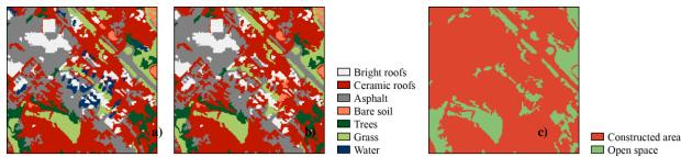
Figure 5 - Post classification process: (a) confusion between water and shadows; (b) corrected classification by conditional thresholds; and (c) merge of the classes corresponding to abstract classes 'Constructed Area' and 'Open Space'.
