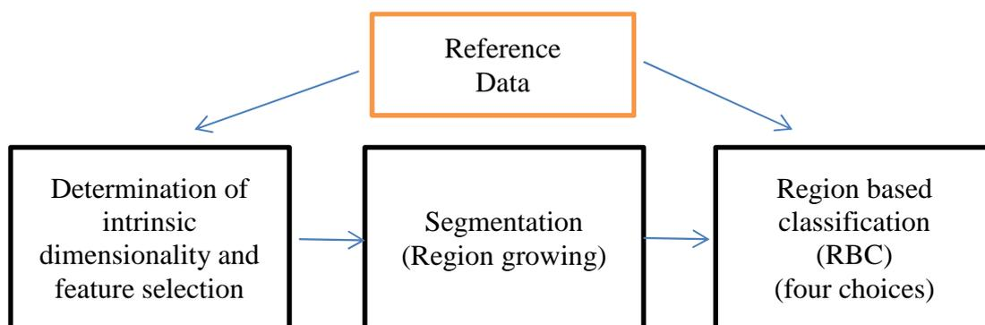
Figure 1: Processing chain for Region Based Classification
