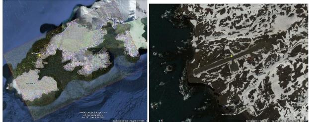
Figure 1. The processed SAR image overlapped on Google Earth® optical image (on the left). Ancillary optical image zoomed on the airdrome area (on the right). The position of the aircraft is highlighted by the yellow pin.
