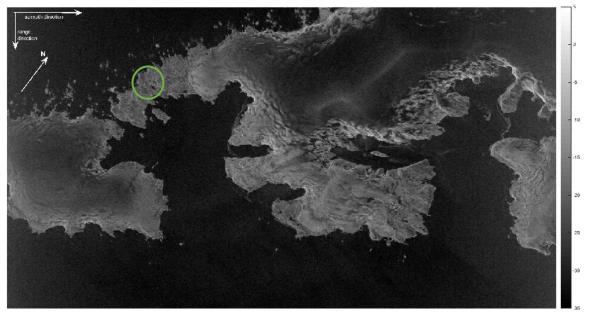
Grey-tone hv-polarized intensity SAR image, in dB scale.
