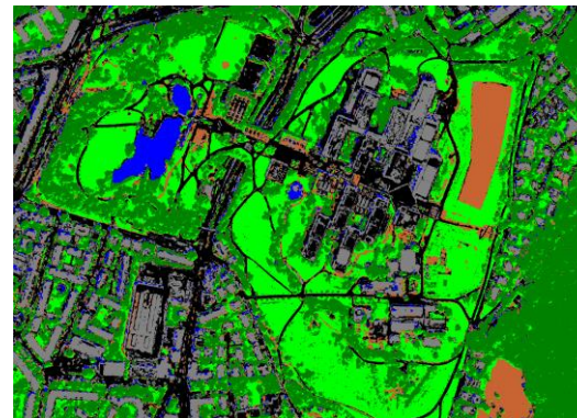
Figure 4. SVM classification result obtained with the RBF kernel ( C = 1; \gamma = 10 ) and the OAO strategy.
