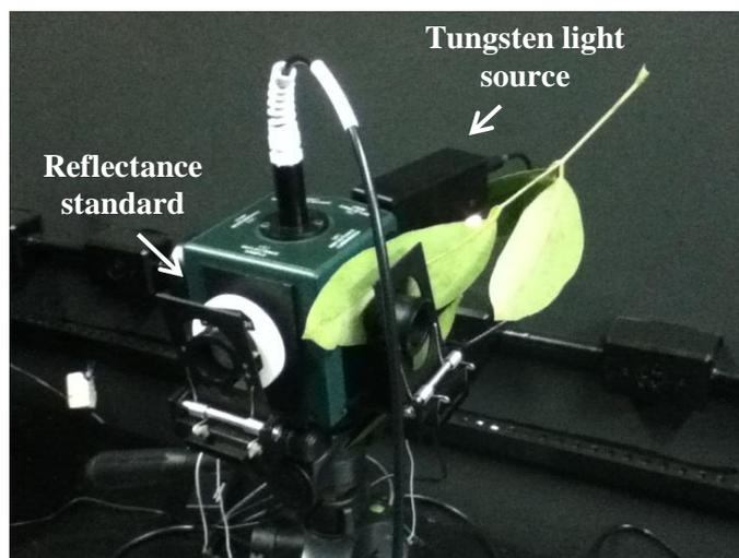
Figure 1. Calibration to leaf reflectance measurement using the ASD/RTS-3ZC integrating sphere.
