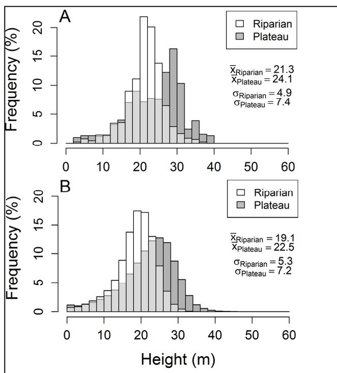
**Figure 5.** Frequency histograms of riparian and plateau forests' top-of-canopy heights at 1m horizontal resolution, from ground LiDAR data (A) and from a Canopy Height Model derived from airborne LiDAR (B).
