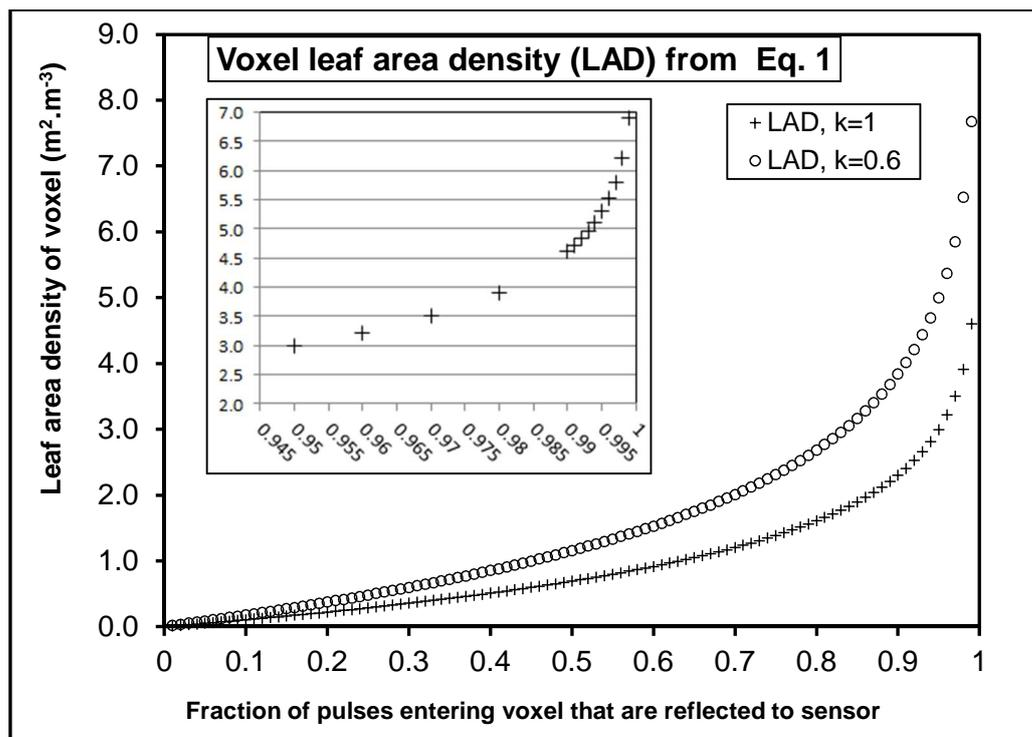
**Figure 2.** Leaf area density estimate of a voxel increases exponentially with the fraction of pulses entering at the base of a voxel that return to the sensor as a last-return distance measurement. Inset shows rapid increase in estimated LAD, when more than 95% of pulses return, for K = 1.
