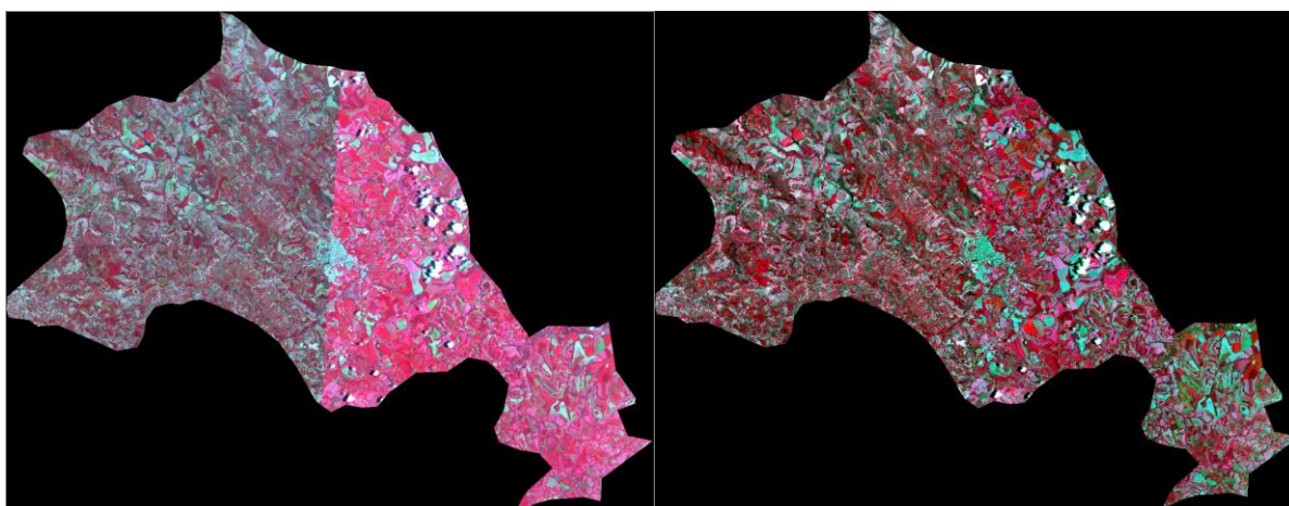
Figure 2. Rapideye images mosaic with no corrections Machado-MG (A) and Rapideye images mosaic with corrections Machado-MG (B).
