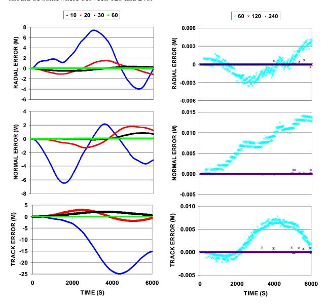
Figure 4. Discrepancies in RNT components for one CBERS satellite orbit with different levels of order and degree truncation
