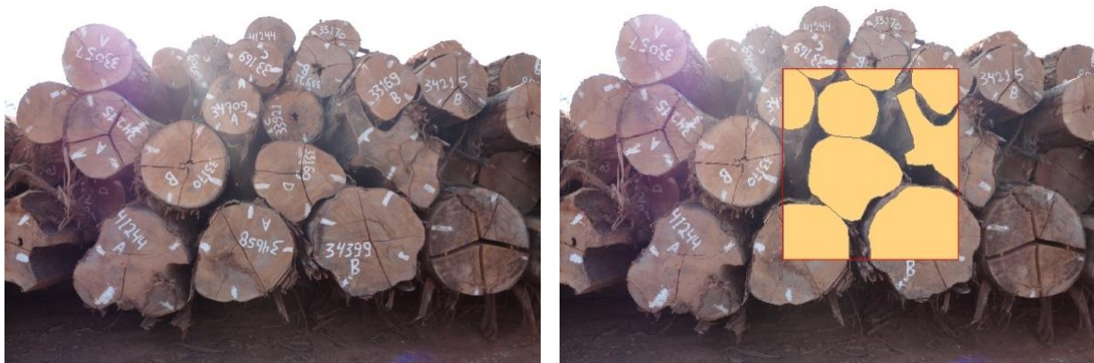
Figure 5 - Example of picture used for determining a stacking factor. The calculation of the stacking factor was made by identifying the log area (yellow polygons) and the empty spaces, inserted into a flat polygon (rectangle with edges in red). For each of the photos, only its most perpendicular portion in relation to the evaluation plan was used.
