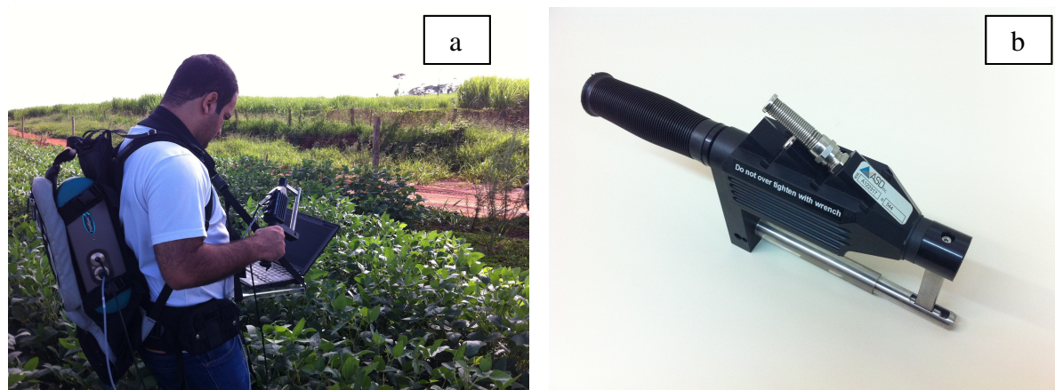
Figure 2. Overview of the procedure for collecting the spectral curves of plants (a) and detail of the ASD Plant Probe (b).
