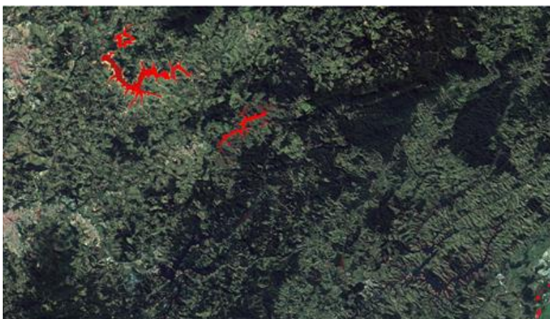
Figure 5. Part of the Jaguari & Jacarei reservoir image in true colour composition (R7 G6 B5) and water is identified (in red) by the select Hue threshold.
