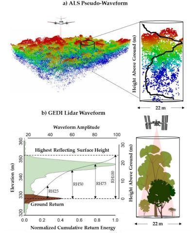
Figure 2. ALS-derived pseudo-waveform (vertical black line) and (b) GEDI-like waveform and canopy metrics.
